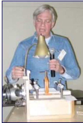
Don Carkhuff— Horizontal router jig.
