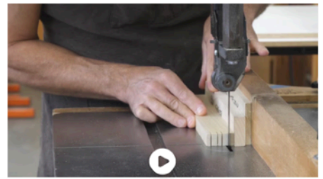
17-How to Machine-cut Double Mortise and Tenons
